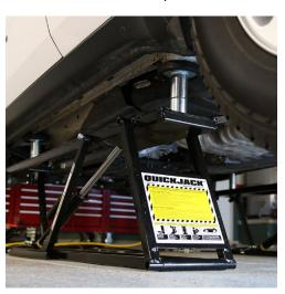
This twelve-piece adapter set increases the service capability of the QuickJack BL-7000SLX and BL-5000SLX series by providing stackable adapters that mount inside the lifting block trays.
